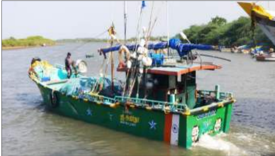
Bottom Trawler converted into Tuna Long Liner
